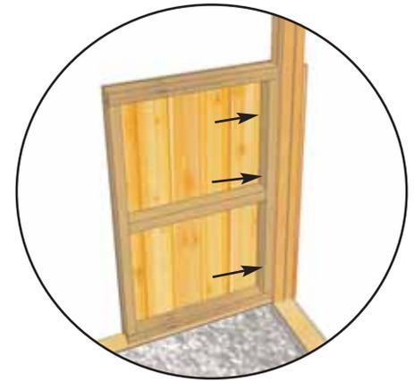
**5.** Position **Part D** (25 1/2" wide Front Solid Wall) even with bottom of Post and with Wall Siding flush with outside of Filler Trim of Post on the outside. Attach with 3 - 3" screws as shown above.
