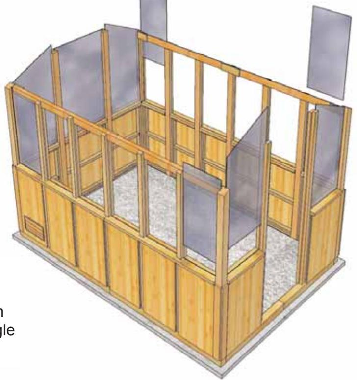
**29.** Make sure the **Window** Slides down into the dado cut of the Top Cap.
