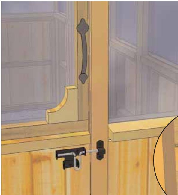
**65.** Attach **Door Handle and Exterior Black Barrel Bolt** to door. Handle is positioned on top door; Barrel Bolt on bottom door. Attach Black Barrel Bolt as illustrated to the left with 3/4" Black Screws.
