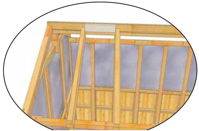
**46.** Install second **Part U - Roof Rafter using Rafter Template Spacer**. Align Spacer tight against Rafter's 2x3 edge. Position Rafter so dado cut of Ridge Board is aligned with gap in Rafter and tight against 2x3 edge of new Rafter. Attach as per **Step 45**.
