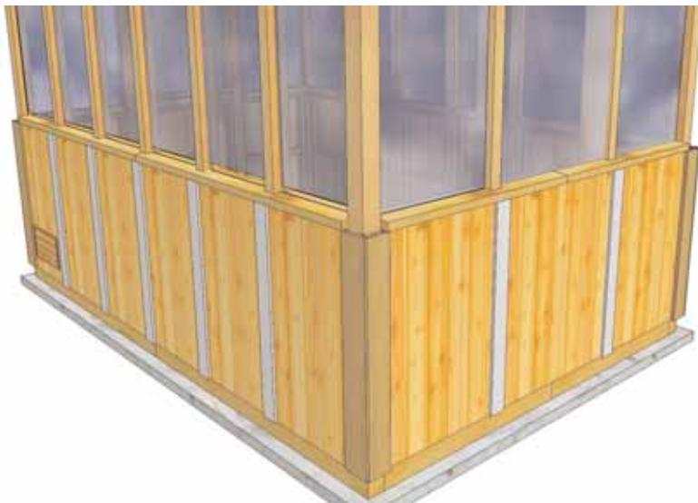
**69.** Locate **Part HH -Vertical Wall Trim - 1/2" x 3 1/2" x 34 7/8"**. Position underneath Top Wall Cap where Walls attach to Posts. Center and attach with 4 - 1 1/2" finishing nails per piece.
