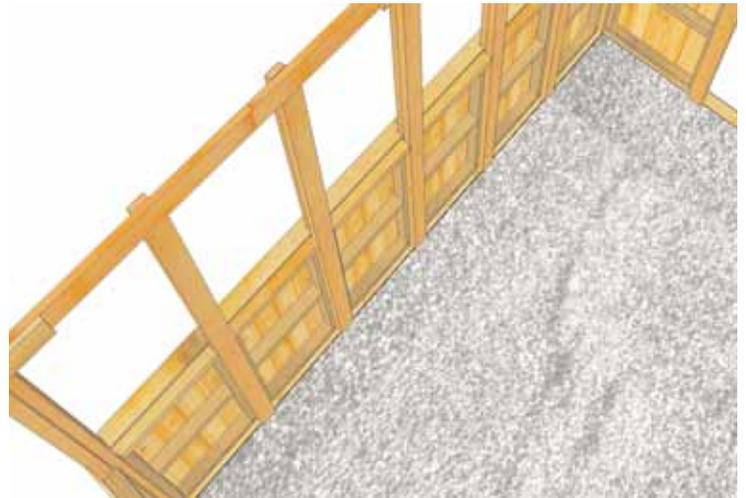
**22.** Complete Side Wall Top Cap on one side. Depending on your footprint measurement, a gap of 1/8" to 1/2" could result where Caps meet in the middle. You may use caulking later to seal the gap.
