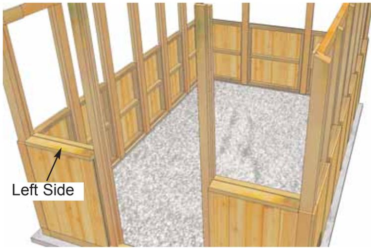
**21.** Repeat **Step 20** to attach Left Side Front Wall Top Cap.
