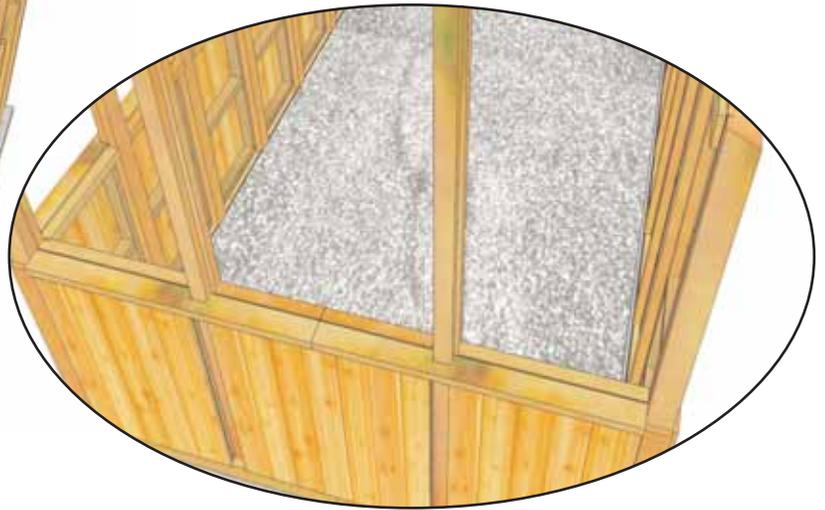
**23.** Locate **Part H - Rear Wall Top Caps - 1 1/2" x 5 1/2" x 44 1/2"**. Position and attach as per **Step 20**. Once again, the Cap is designed with tolerance and gaps will appear around the notches. Later, caulking may be applied to seal these gaps. Complete remaining Side Wall Top Cap attachments as shown to the left.
