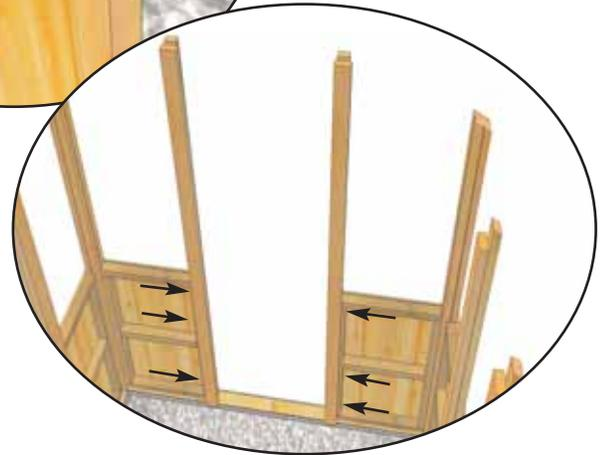
**13.** Locate **Part I.** The Doorway / Wall Framing Sets. There are 2 Sets (Front/Rear). Align and install Vertical Posts from the set as per **Step 9.** Install rear side first. (Vertical Posts are not shown correctly. They have angle cut on one end.)
