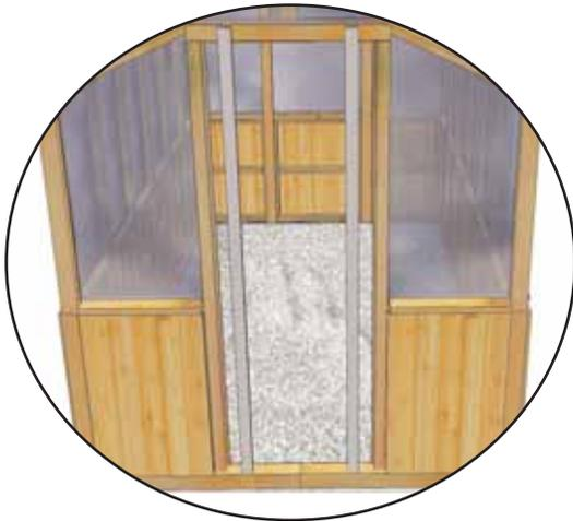
**60.** Locate **Part CC & CCC - Vertical and Horizontal Door Filler Trim - 3/4" x 2 1/2" x 33" & 87 1/4" long.** Position 3/4" Vertical Filler Trim on Doorway Framing and attach with 6 - 1 1/2" finishing nails. There are two pieces.
