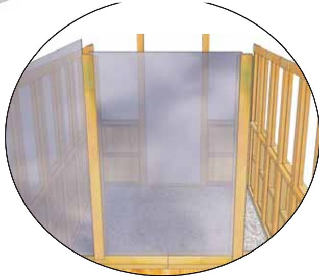
**26.** Locate **Part L - Rear Center Polygal Window - 33 3/4" wide**. Once again, peel protective plastic layer off first and note correct side out. On a step ladder, lift window up and position between gap of Doorway Posts. Slide down and position as per **Step 25**.
