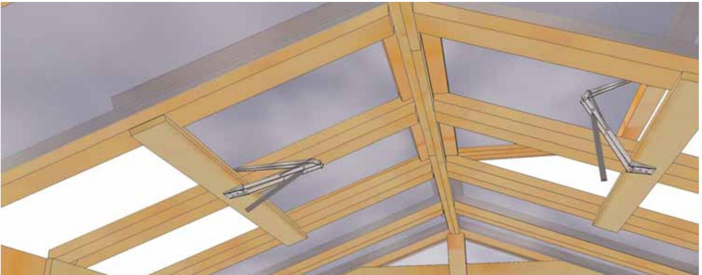
**Important-** Heat Activated Hinges will open only after the Greenhouse reached an inside temperature of approximately 75 degrees Fahrenheit. Make sure Hinged Windows open easily and do not stick. We recommend purchasing a thermometer once the Greenhouse is complete. Please monitor Heat Activated Hinges to confirm they open and are functioning correctly.
