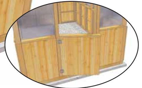
**63.** Locate **Part AA - Bottom Dutch Door - 32  $\frac{1}{2}$ " x 35  $\frac{1}{2}$ "**, **2 - Black Butt Hinges** and **12 - 2" Black Screws**. On ground, attach Hinges to Door first using 2" Black Screws. Align/shim Door and attach to Door Trim with 2" Black Screws. Confirm Door swings correctly before attaching all screws.
