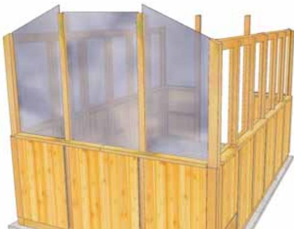
**27.** Locate a second **Part K - Outside Angle Cut Polygal Window - 26 1/2" wide**. Position as per **Step 24-25**.
