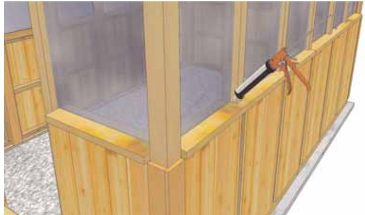
**44.** Once all Side Windows are installed. Caulk Window / Wall Top Cap seam. Work around the entire Greenhouse. Gaps in Wall Top Caps can also be caulked at this time. No need to caulk sides or top at this time.
