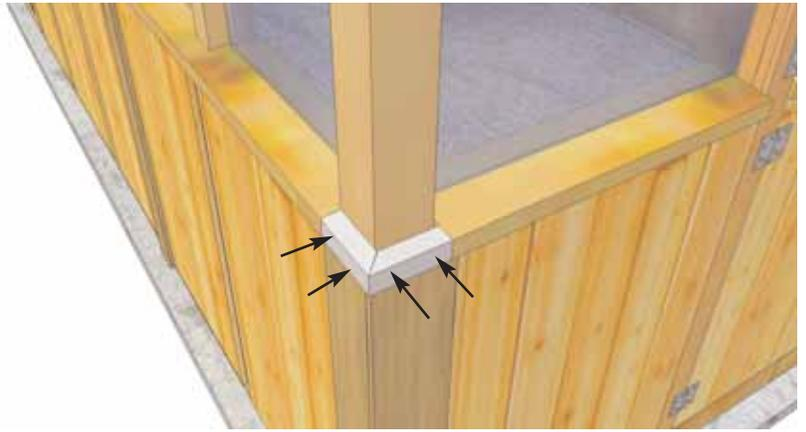
**70.** Locate **Part II - Corner Post Trim - 1 1/2" x 1 1/2" x 5"**. Position around each Outside Corner Post. Attach with 2 - 2" finishing nails per piece.
