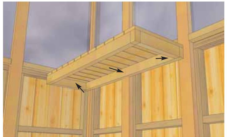
**74.** Locate **Parts MM and NN - Potting Shelves - 16" x 45 3/8"** and **Potting Shelf Supports - 1 1/2" x 2 1/2" x 20 1/2"**. With helper holding Shelf just under the Top Wall Cap, screw to wall from underneath with 3 - 3" screws as shown above.
