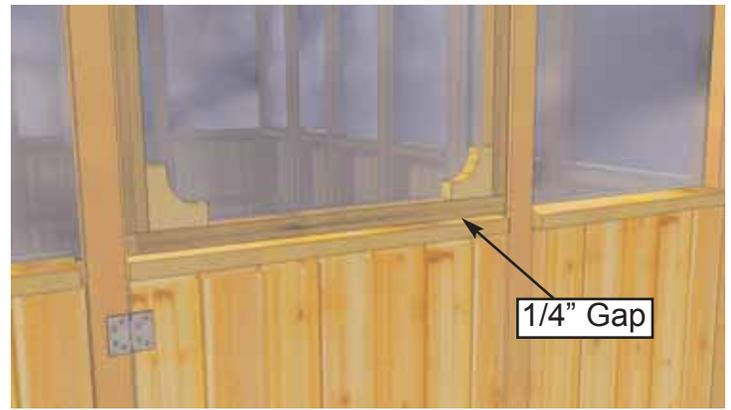
**64.** Locate **Part BB - Top Dutch Door - 32 1/2" x 47"**, **2 - Black Butt Hinges** and **12 - 2" Black Screws**. On ground, attach Hinges to Door first using 2" Black Screws. Align/shim 1/4" from Bottom Door and attach to Door Trim with 2" Black Screws. Confirm Door swings correctly before attaching all screws.
