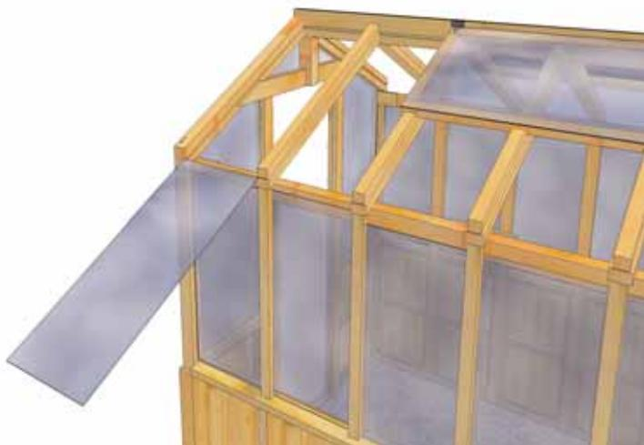
**51.** Locate **Part X - Roof Polygl Windows - 21" wide x 51" long**. Peel protective plastic layer off first sheet noting correct side out. Fit Window in dado of Outside Rafter and gap of inside Rafter as shown above.
