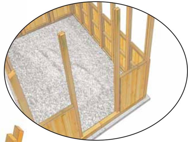
**15.** Install the Vertical Posts from the Front Set of **Part G**, as per **Step 14**.
