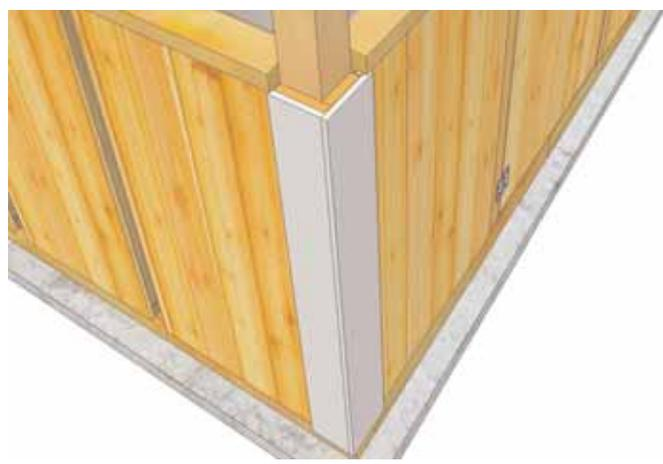
**67.** Locate **Parts FF & GG - Outside Post Trim Narrow- 1/2" x 4 1/2" x 34 7/8"** and **Outside Post Trim Wide - 1/2" x 5 1/2" x 34 7/8"**. Position with Wide Trim capping the side when looking at the front. Align Trims so flush under Wall Top Caps and attach with 4 - 1 1/4" finishing nails per piece.
