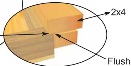
**9.** Position Post R against Wall Framing as shown above. Make sure Post is flush with bottom of wall framing. Locate Temporary Post/Wall Supports (3" high) and place underneath 2x4 edge and touching 2x3 as shown above. Clamp and attach Post to wall framing with 3 - 3". Do both sides.
