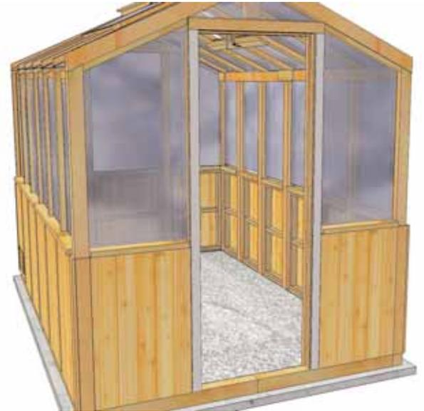
**62.** Locate **Part DD & EE - Vertical & Horizontal and Vertical Door Trim -  $\frac{1}{2}$ " x 2  $\frac{1}{2}$ " x 38"** & **84  $\frac{1}{4}$ "**. Position  $\frac{1}{2}$ " Thick Horizontal Trim over Horizontal Filler Trim and attach with 4 - 1  $\frac{1}{2}$ " finishing nails. Position  $\frac{1}{2}$ " Thick Vertical Trims over Filler Trims and attach with 6 - 1  $\frac{1}{2}$ " finishing nails per piece.
