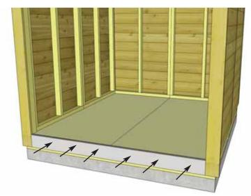
**48.** Position **Front Skirting** (3/4" thick) between Door Trims aligning it even at top edge with floor. Use 6 - 1 1/2" nails to secure.
