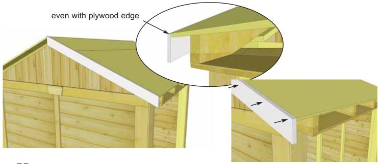
**55.** Locate **Side Facia** (angle cut on both ends). There are 2 left and 2 right side pieces. Correct positioning is rough side out. Starting on one side, line facia up so the end is even with edge of plywood roof. Attach to plywood edge with 8 - 1 1/2" nails. Align 2nd Side Facia piece up with plywood edge. Note that there will be a slight gap where facias meet at the peak. This will be covered up with the Pentagon Facia Plate in Step in **Step 57.** Attach with 8 1 1/2" nails.
