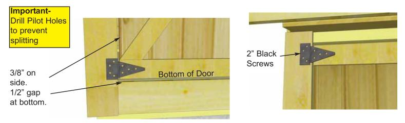
**60.** With Door correctly aligned, attach Door Hinge to Door Trim with 2" black screws. **Hint:** Do not attach all the 2" screws in each hinge until both doors are positioned correctly into place. Drill pilot holes in Door Trim prevent wood from splitting. When satisfied with door positioning, complete all 2" screws then.
