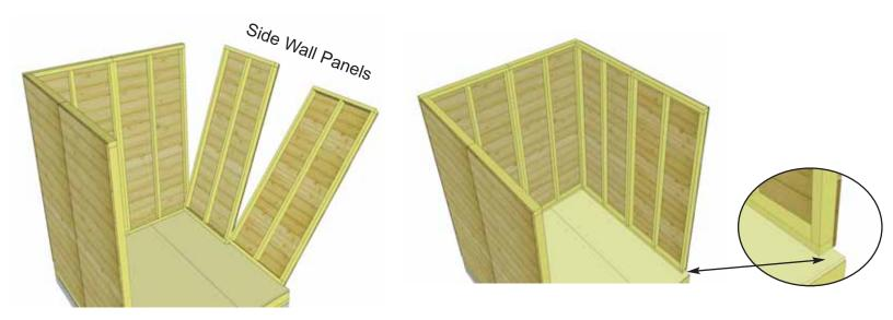
**20.** Position and attach remaining side wall panels together as per **Steps 16-18**.
