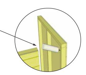
**16.** Position side wall into place on plywood floor. Butt both vertical wall studs of side and rear walls together and attach with 3 - 2 1/2" screws. Screw at the bottom, middle and top of stud to secure properly.
