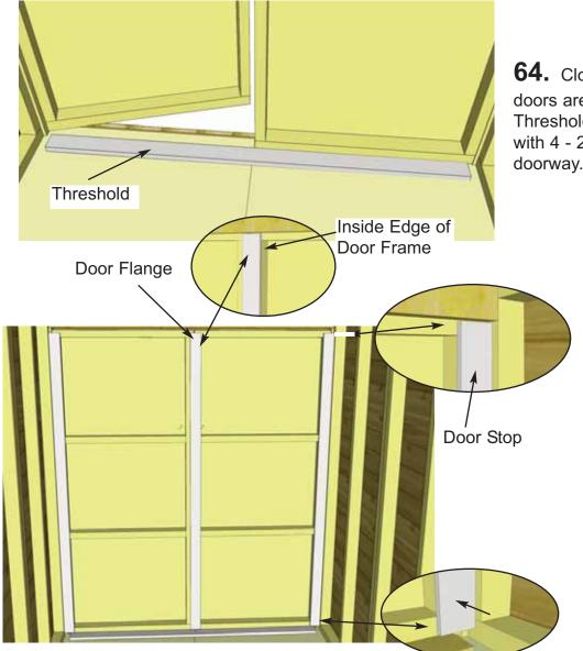
**64.** Close both doors and align so doors are straight. Attach Door Threshold (2 1/2" wide x 62 1/2" long) with 4 - 2" screws centering between doorway.
