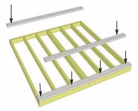
6. Attach Floor Runners to completed floor frame. There are 3 floor runners per 70" side. Use 8 - 2 1/2" screws per Runner.
