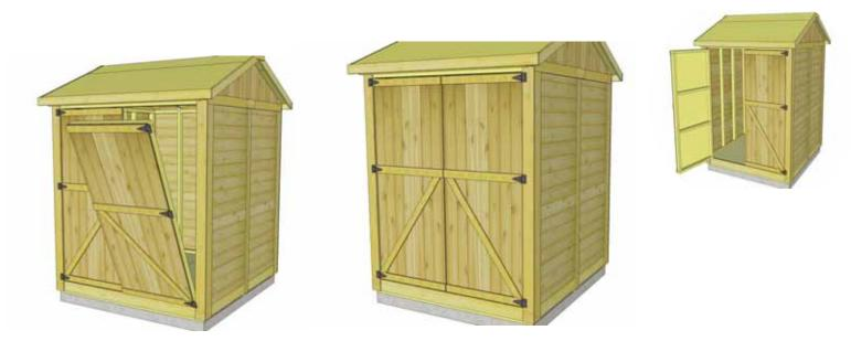
**61.** Position and attach **Right Side Door** as per **Steps 59-60**. Door position may need slight adjusting to open and close correctly. When satisfied, complete all 2" screws. **Note**, Do not over tighten hinge screws when using screw gun.
