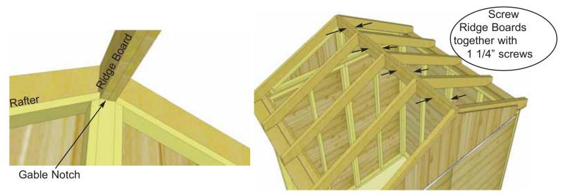
**39.** With Ridge Board locked into gable notch, align Ridge Boards so they are flush together and secure them with 8 - 1 1/4" screws. **Important**- if there is a gap between Ridge Boards, try pushing rear wall and Door Header closer together from outside. Walls should be 70" apart at top from inside of wall plate to wall plate.
