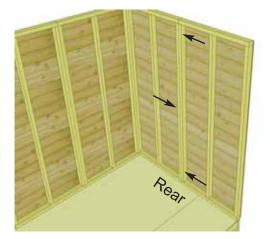
**19.** Align wall panel framing flush with floor framing and attach vertical wall studs together as per **Step 18**.
