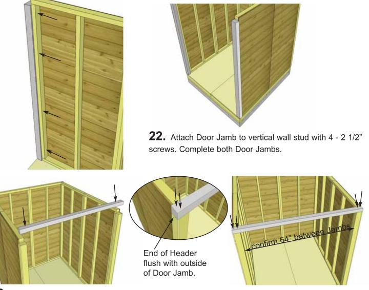
**23.** Position and attach the Door Header flush to outside end of Door Jamb with 2 - 2 1/2" screws per side. Important- Drill 1/8" pilot holes in end of Door Header to prevent wood from splitting.
