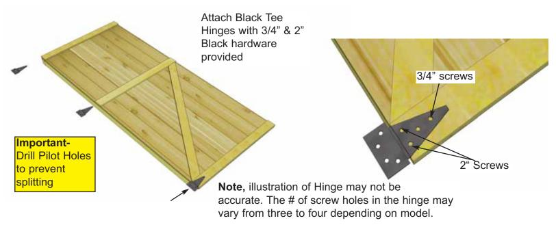
**58.** Attach Door Hinges to both **left** and **Right Side Double Doors**. Position Hinges equally on door trim as shown above and attach with Black 3/4" and 2" screws.
