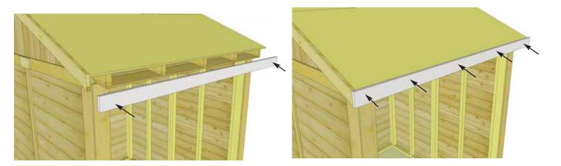
**56.** Position and attach **Front Facia** to ends of Roof Rafters with 10 - 1 1/2" nails. Front Facia will cap side facia in corners and line up on top edge with plywood roof.
