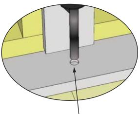
Drill 1/2" Diameter Hole to accommodate rod of Cane Bolt.
