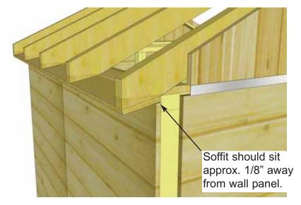
**37.** When Rafter Section is correctly positioned, outside rafters will sit equally on gable framing and Soffit will sit approximately 1/8" away from wall panels.
