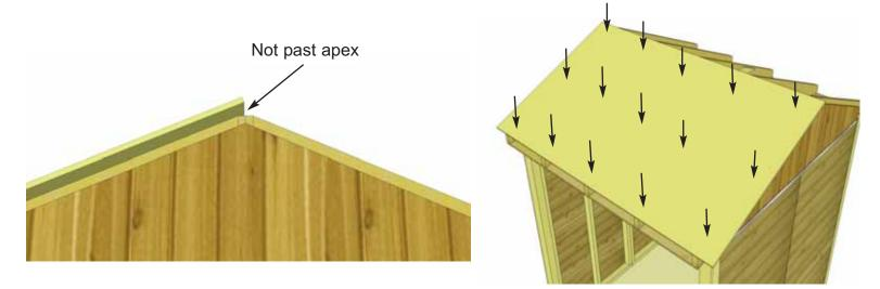
**44.** When Plywood is correctly positioned, fasten down into Roof Rafters with 15 - 1 1/4" screws.
