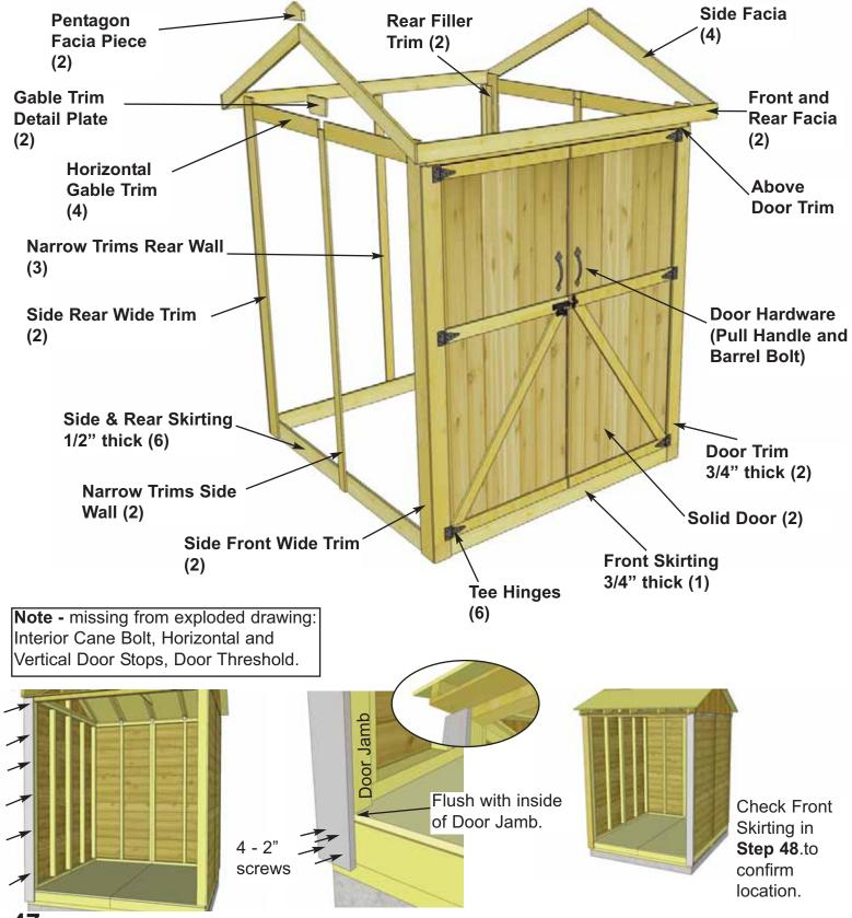
**47.** Locate both 3/4" x 4 1/4" x 79" Door Trims. Position a Trim so it covers the Door Jambs and is flush with the inside of it. Secure with 6 - 1 1/2" finishing nails. At the bottom, use 4 - 2" screws. Complete both Door Trims. **Important- Drill 1/8" pilot holes in bottom of Door Trims to prevent wood from splitting.**
