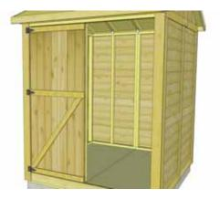
**59.** Next, position and secure the Double Doors. Starting with **Left Side Door**, position so there is a 1/2" gap on bottom and approximately 3/8" on the side. Use a spare Shingle to shim door in place at the bottom.
