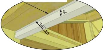
**63.** Position Horizontal Door Stop with dado facing out, tight against Door Header. Align so Dado cut is flush with Header leaving approximately a 1" overhang in the doorway. Attach with 6 - 2" screws.
