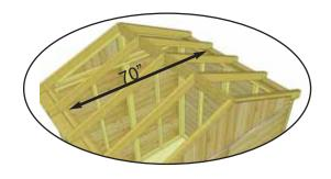
41. Secure Rafters to Top Wall Framing with one 3" screw per rafter. Screw through Wall Frame at an angle. Have two helpers push the Front and Rear Walls at the top from the outside of shed until inside to inside measurement between the Top Plates is 70".
