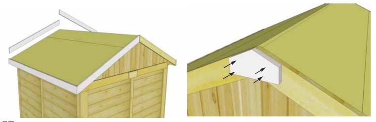
**57.** Complete remaining facia pieces. Attach **Pentagon Facia Plate** where Side Facia meet at the peak. Use 4 - 1 1/2" finishing nails per piece to secure.
