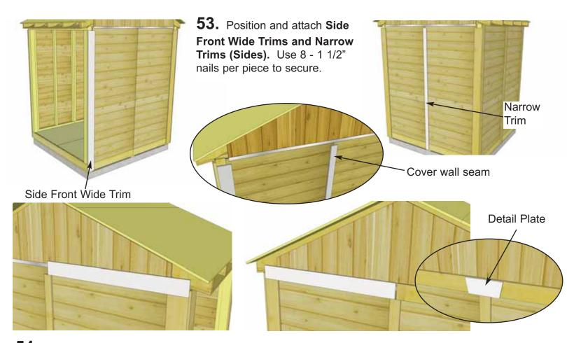
**54.** Attach Horizontal Gable Trim ( 4- 1/2" x 4 1/2" x 37 7/8") to both sides of shed. (2 per side). Position over gable and wall seam. Use 4 - 1 1/2" nails to secure each piece. Make sure gable trims covers flashing completely. Align even with outside of wide trim leaving a slight gap a center. Attach Horizontal **Detail Plates** over Gable Trim seam and secure with 4 - 1 1/2" nails. Complete both sides.
