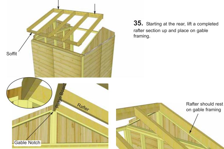
**36.** Slide Rafter Section up on gable framing until bottom of Ridge Board slips into gable notch.
