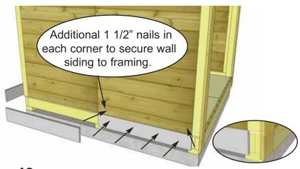
**49.** Attach **Side and Rear Skirting** around the base of the shed. Skirting will hide floor framing. The side skirting pieces will meet together in the center. Gaps on outside will be covered by Wide Trim pieces later. Use 4 - 1 1/2" nails to secure. Further secure bottom siding to wall framing in corners on each wall panel with 2 - 1 1/2" nails.
