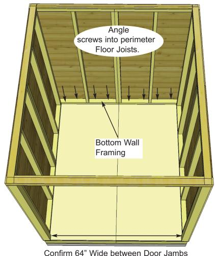
**27.** When all Walls and Top Plates are attached together, check wall and floor alignment. Bottom wall framing should sit flush with outside of floor joists. See **Steps 15-20** for correct alignment.
