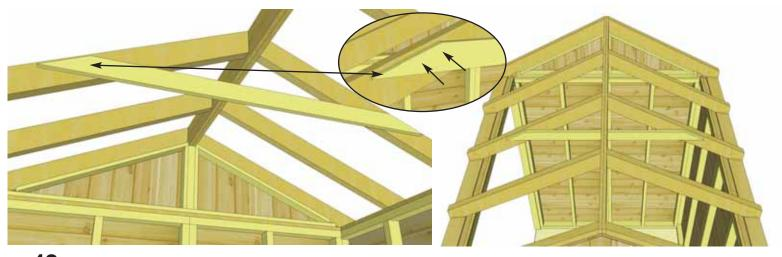
42. The Roof Gusset is positioned on center rafter. When correct, slide gusset up, use level to square gusset and attach to rafter with 4 - 1 1/4" screws. Pilot hole Gusset to prevent splitting.
