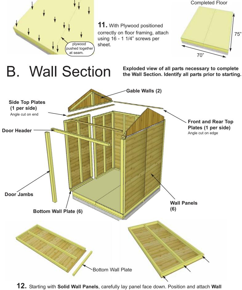
**12.** Starting with **Solid Wall Panels**, carefully lay panel face down. Position and attach **Wall Plate** to bottom of wall studs of each wall panel with 3 - 2 1/2" screws. Position plates flush with framing.
