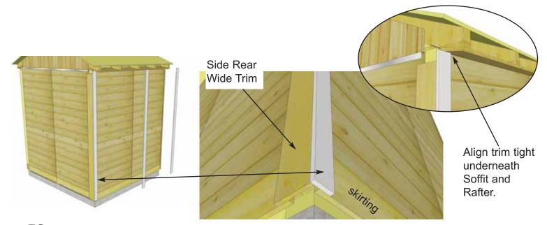
**52.** Attach **Narrow Trims (Rear Walls)** to in each rear corner and middle wall seam (3 - 1/2" x 2 1/2" x 79"). Use 8 - 1 1/2" finishing nails per piece. Align Trims tight underneath Soffit and Rafter and so it caps the Side Rear Wide Trim.
