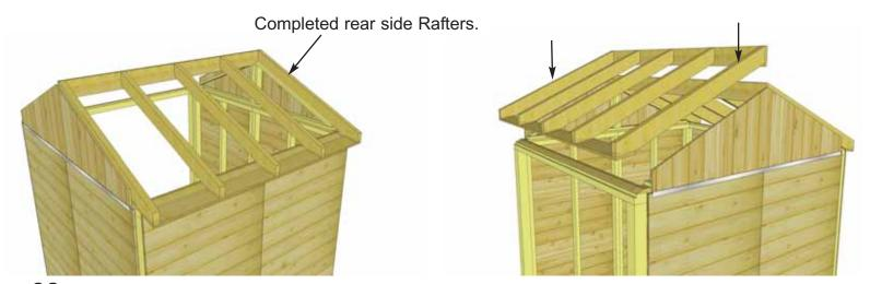
**38.** Place 2nd completed Rafter Section on gable wall framing. Position as per **Steps 34 - 36.**
