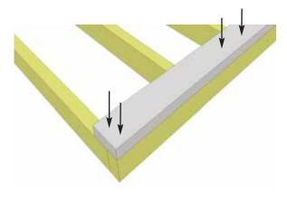
7. Make sure Runners are flush with outside and front and rear floor framing but not overhanging.
