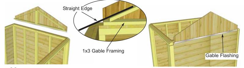
**28.** Place Gable so framing sits flush with the inside of the top plate. Center from front to rear using a Straight Edge to confirm angle of gable frame and Top Plate line up. Adjust gable accordingly. From the outside, make sure gable flashing overhangs wall siding.
