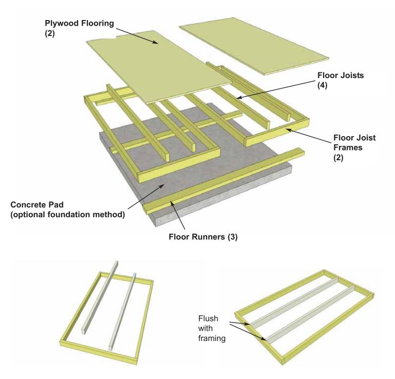
**1.** Lay out one **Floor Joist Frame and 2 Floor Joists** as illustrated above. Position Joists equally in Floor Joist Frame. Position Joist so flush with framing.
