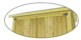
**62.** Place **Above Door Trim** on door header between door trims. Attach with 6 - 1 1/2" nails. Leave small gap to allow for proper door opening and closing. Hor. Door Stop with Dado cut.
