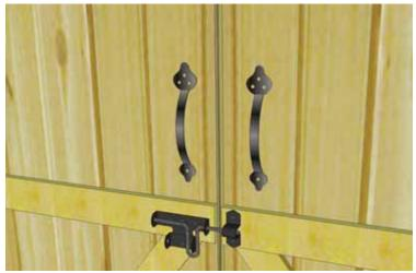
**68.** Attach **Door Handles.** Handles are positioned on top section of each door and mounted with 3/4" Black Screws.
