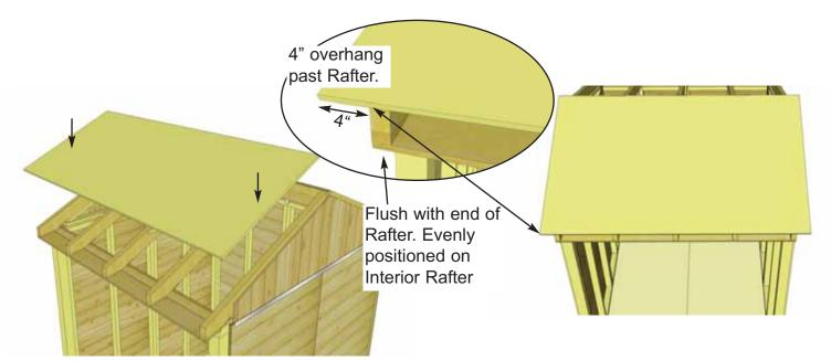
**43.** Starting in front corner, !scate 5/8" x 78" x 45 1/4" Plywood Roof Section and place on top of Roof Rafters. Position so Plywood overhangs outside Rafter by 4". At bottom of Rafter, Roof Panel should be flush with Rafter end.
