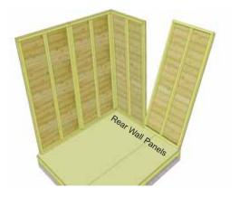
**18.** Align vertical wall studs of both side wall panels together and attach with 3 - 2 1/2" screws. Wall siding should overhang floor by approximately 1/2". Position 2nd rear wall panel as previously described.
