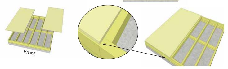
**10.** Position **Plywood Floor** pieces (2) on top of completed floor frames. The Plywood is cut slightly smaller than floor framing. Keep plywood seams tight.
