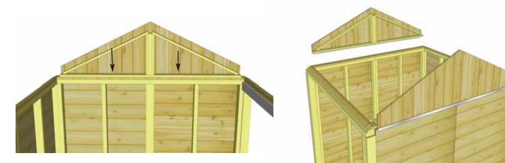
**29.** Temporarily attach Gable to walls and top plate with 2 - 2" screws. Screw from the bottom of gable framing down into Top Plate and Wall. Gables may need slight adjustment in **Step 40** and then be completely attached with an additional 6 - 2" screws. Position 2nd Gable on side walls.
