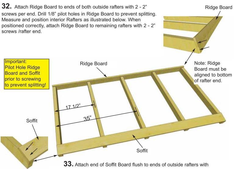
2 - 1 1/4" screws per rafter end. Drill pilot hole in Soffit ends to prevent splitting. Complete both outside Rafter / Soffit connections first. Measure and position interior Rafters as illustrated above. When positioned correctly, attach Soffits to remaining rafters with 2 -1 1/4" screws /rafter. Flip completed rafter section over.
