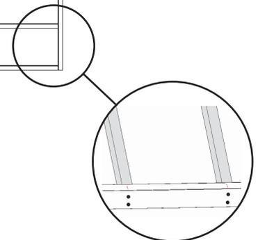
Place the 2" x 4" x 120 1/2" boards on the inside of the frame. Nail each board in place with the 16d nails.
