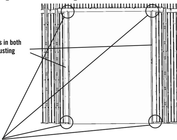
Loosen these Carriage Bolts before adjusting Doors.
