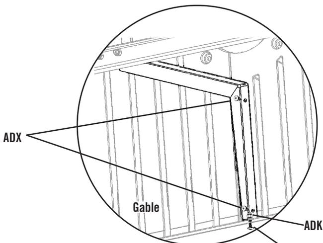
There are no pilot holes in the Gable to receive the Screws (ADX). Insert them directly into the plastic.
