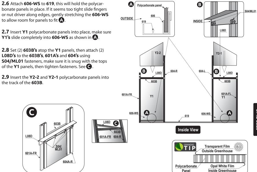
2.10 Move roof and front section together and align the WG02's into the 601A's, and align the S04/ML01's on the W02T's into the 604's. Insure a snug fit between the W02T's, 601B's and 601A's and then tighten the S05 screws as shown in A. Tighten the W02T's with the S04 /ML01 nut and bolt as shown in B.
