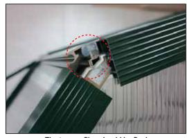
The two profiles should be flush at ends when installed correctly.
