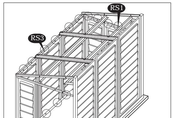
3. Attach each side panel (SP↑) on top to the roof structure (RS1) and (RS3). Using a dia. 3mm (1/8") drill with a power drill, make two equal distance holes on the side panel through the roof structure. Drive a self tapping screw (S4) through the side panel to the roof structure. Repeat this for every side panel. See blowup.
