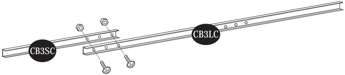
8. Assemble the center bands (CB3SC) & (CB5C) with (S3) screws with nuts. Fix (FCB5C) to (CB5C) with (S3) screws with nuts. Follow overlapping method shown below.
