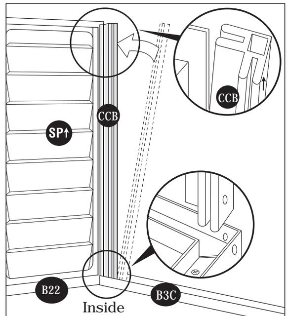
11. Working outside Use (S1) screws to secure column to bases (B22) and (B3C).
