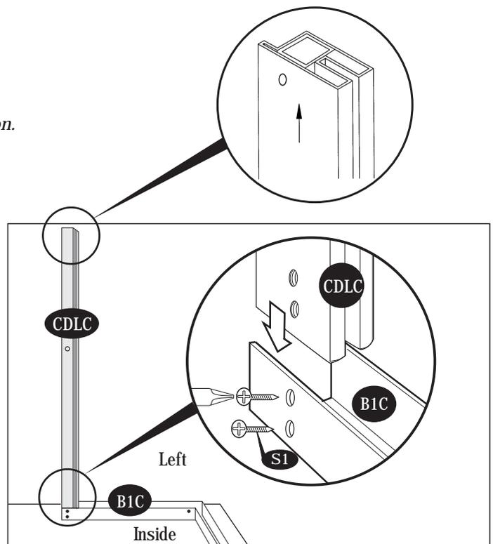
2. Insert the front side panel (FSP↑) into the groove of column (CDLC). Start at the bottom of the panel at an angle then push into place.
