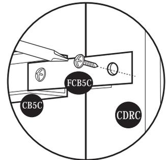
Fig.4: Use (S1) screw. Fix (FCB5C) to (CDRC).
