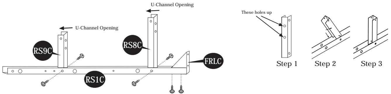
10. Assemble roof structure (RS2BC) to (RS8C) & (RS9C) with (S1) screws.
