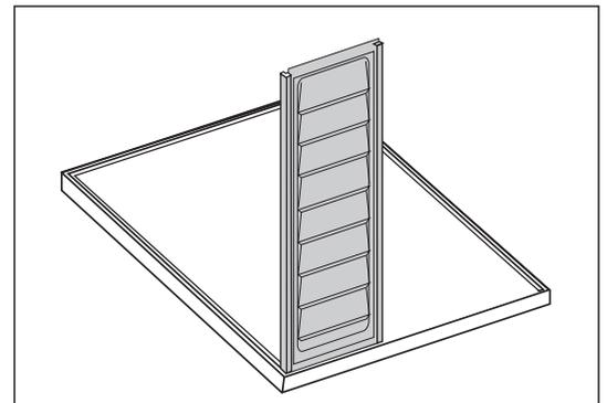
7. Assemble the center bands (CB3SC) & (CB3LC) with (S3) screws with nuts. Follow Overlapping Method shown below.
