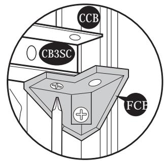
Fig.5: Use (S1) Screws. Fix (CB3SC) to (FCB) fitting.
