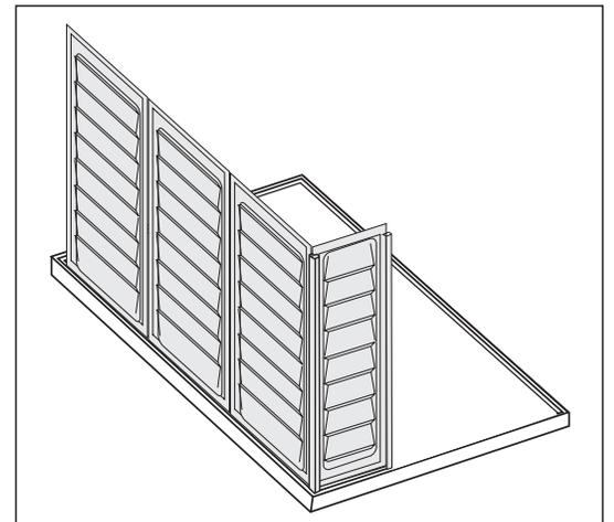
13. Working from inside continue connecting the side panels (FSP↑) and (SP↑) with columns (CMB) in sequence along (B3C) base. Use (S1) screws to fix columns to base.
