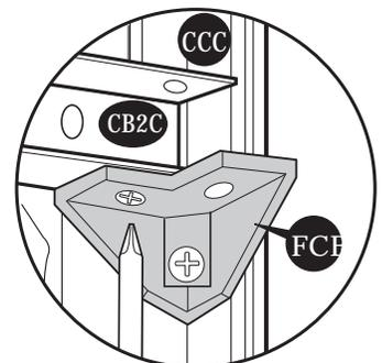
**Fig. 4:** Use (S1) screw. Fix (CB2C) to (FCB).
