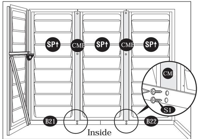
10. Slide corner column (CCB) into side panel (SP↑) pushing the column to the side panel.
