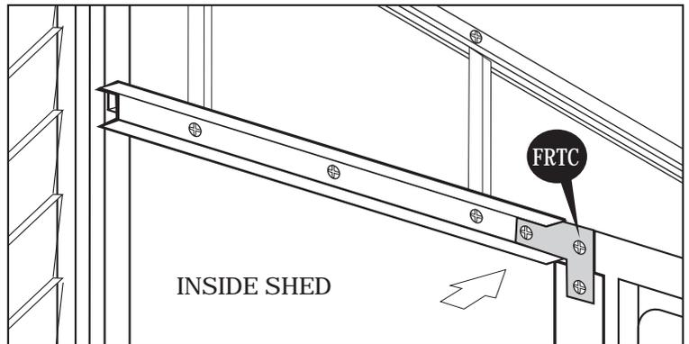
22. Attach center band (CB6C) to door column (CDLC) and 90 degree joint (R.J).
