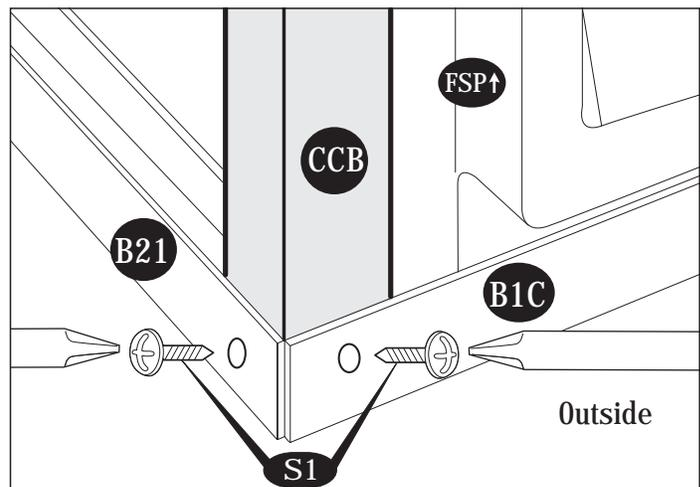
**5.** To stabilize the front panel attach the front center band (CB1C).
