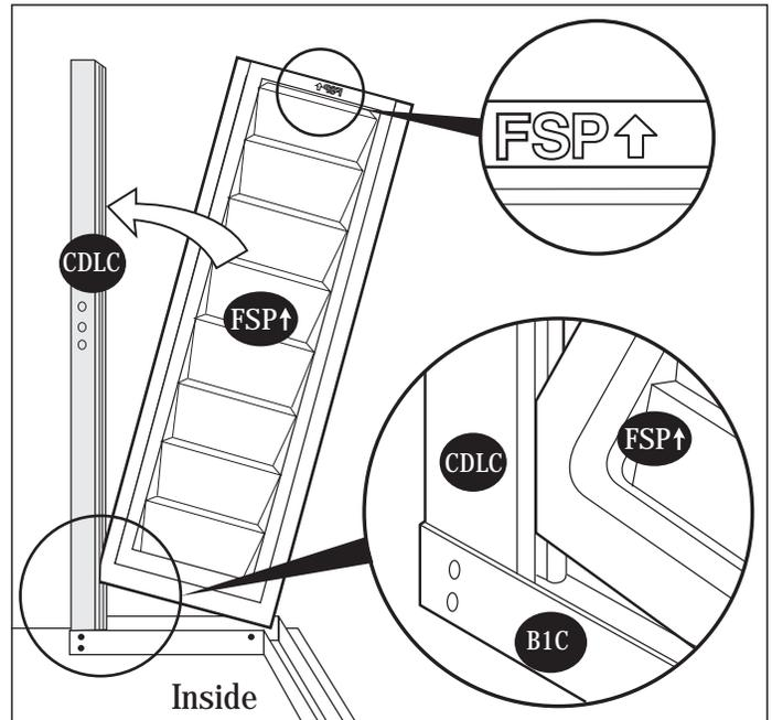
3. Slide corner column (CCB) into side panel (FSP↑) pushing the column to the side panel.
