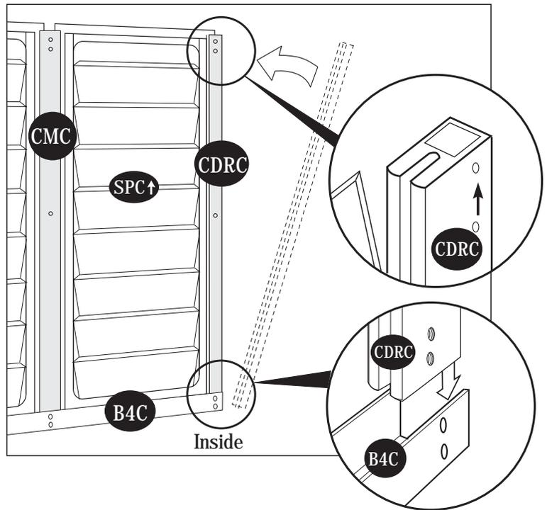
19. Working from inside use (S1) screws to secure the door column (CDRC) to base (B4C).
