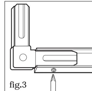
12. Assemble the roof structure (RS5C) into (RS6C) with 6 (S3) screws with nuts (2 sets).
