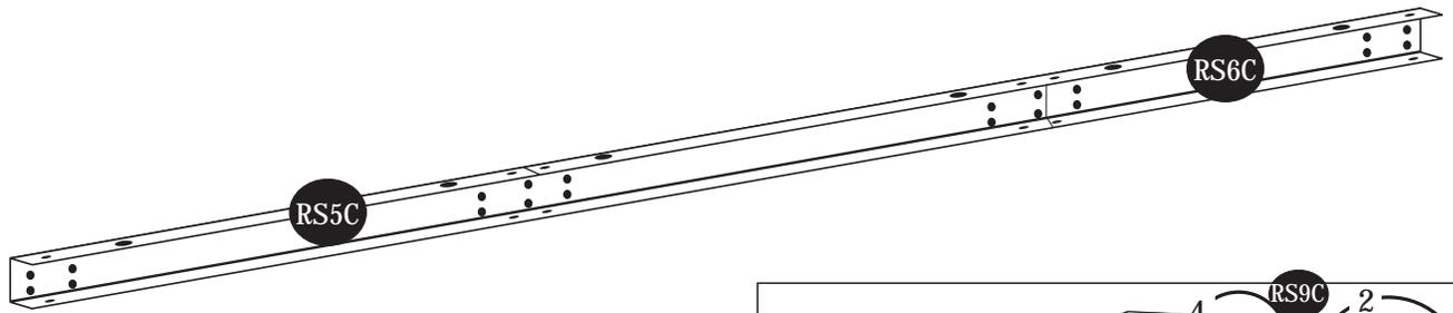
**14.** Place the roof structure assembly (RS5C) with (RS6C) into position on roof supports (RS8C).
