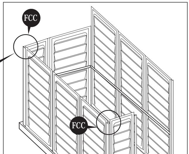
3. Insert the door column fitting (FDCLC) into the door column (CDLC) square tubing inserts.
