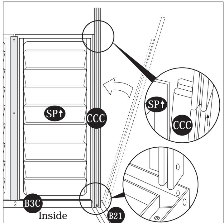
15. Working from outside use (S1) screws to secure the corner column (CCC) to bases (B3C) and (B21).
