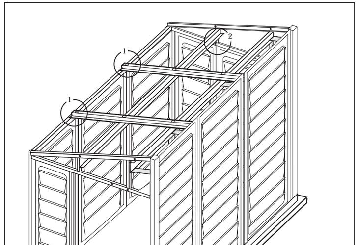
**19.** Fix 'L' bracket (FRLC) to the columns with (S1) screws. See (fig.1)
