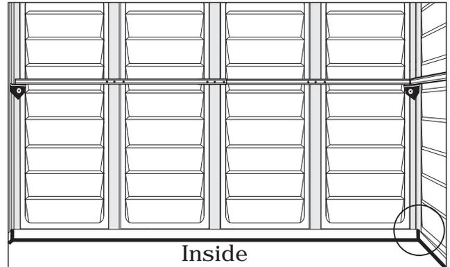
2. After completing the panel assembly, apply silicone around the roof plugs. This is optional and should be done for heavy rain areas if needed.
