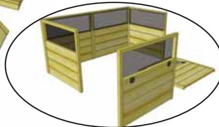
**6.** Align and attach Front Panel - **Part B** to Side Panel with 3 - 2 1/2" . Align panel framing together as **Step 2**. Screw only into Front Panel framing below the screen hinged top.
