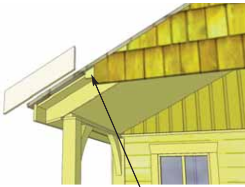
exposed plywood of gable
